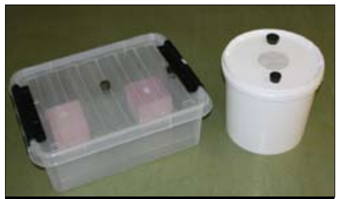
Picture 3: Boxes used for testing of insulations ability to withstand carpenter ant ( Camponotus ligniperda ) nest excavation
